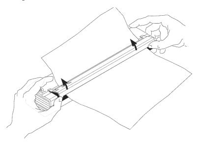
Figure 15. Opening the release cover
